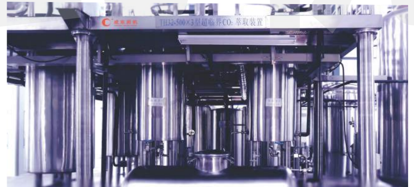
菏泽尧舜牡丹生物科技有限公司TH32-500X3型超临界CO 2 萃取装置 Heze Yaoshun Peony Biotechnology Co.,Ltd. TH32-500X3 Type CO 2 Supercritical Fluid Extraction Device
