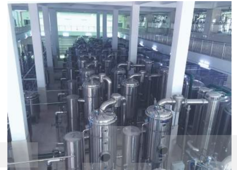
双效自动浓缩系统 Double effect automatic concentration system
