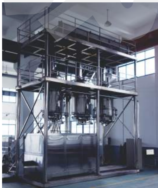
中药数字化自动投料、出渣提取生产线(流程样机) Digital automatic feeding and dreg discharging chinese medicine extraction production line (system sample machine)
